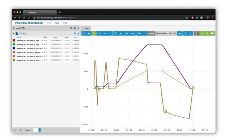
PowerSpy is a graphing tool, targeting the needs of power converter experts at CERN. It can display analogue and digital time-series signals, text data and CERN power converter event logs. While it was developed for CERN, it could certainly be of interest to power converter experts at other labs.
